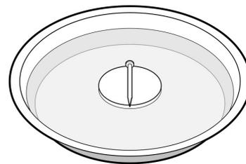
**STEP 2.** Now make a **rubbed** nail as follows. Far away from the floating nail, pick up a second **unrubbed** nail and hold it horizontally at its head end. (The end you would hit with a hammer.) Pick up the bar magnet, hold it at right angles to the
